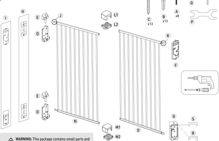
Ensure the surface you are mounting the gate to is structurally sound, such as solid timber, brick or masonry. For plaster/gyprock surfaces, locate the timber beam or stud behind the wall and mount in this location (mounting on plaster/gyprock alone is not strong enough and not safe). Do not mount to glass.
